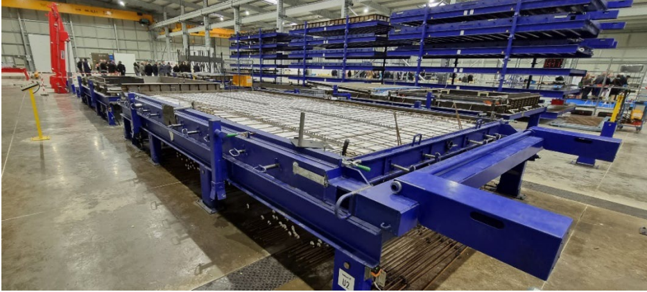
Image 3: The 3D modular concept works with a combination of prestressed solid floors, load-bearing interior walls and columns and insulated sandwich exterior walls.
