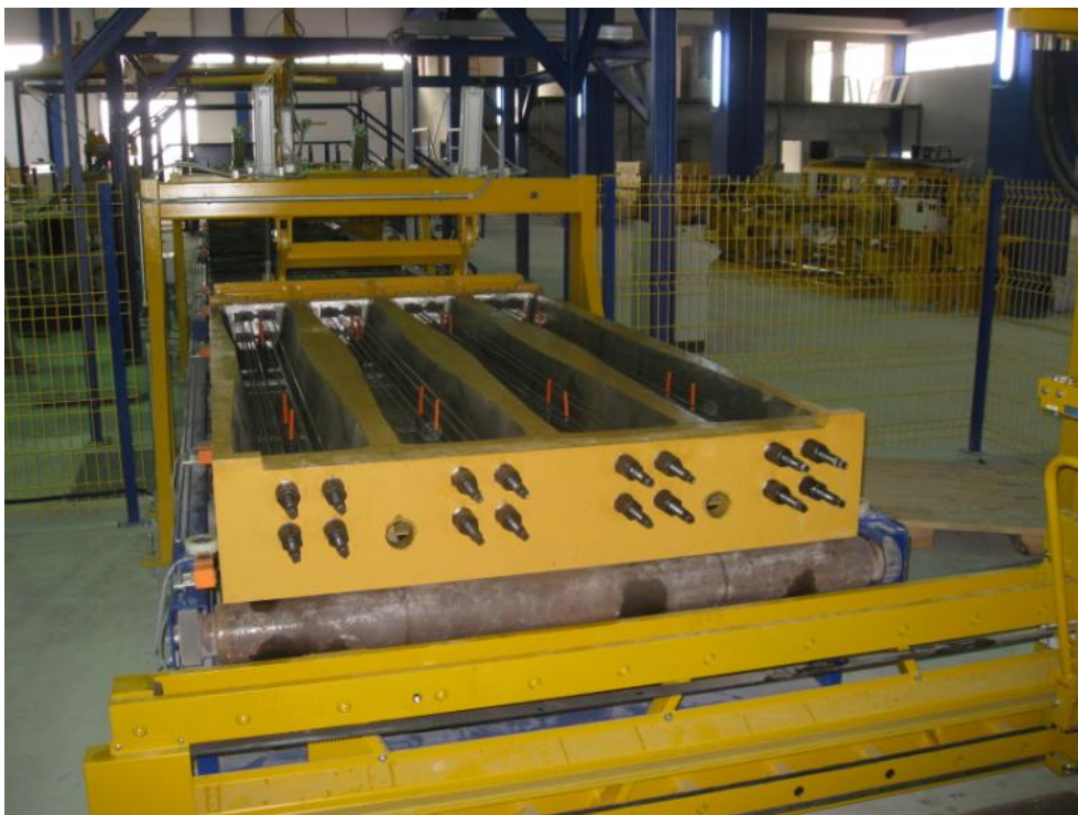
Fig 2: Sleeper form after bringing in the reinforcement
