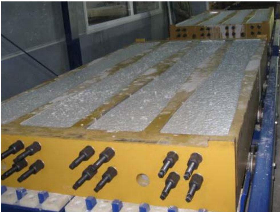
Fig 4: Sleeper form after concreting
