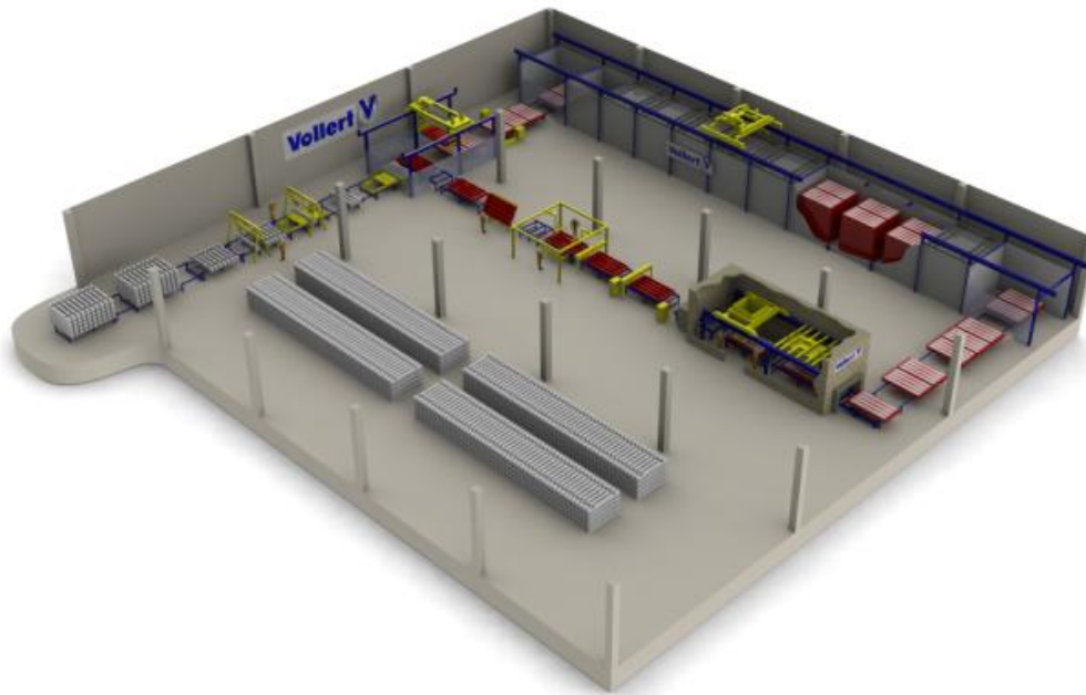
Fig 1: Production plant for up to 450.000 pre-stressed concrete sleepers in a year
