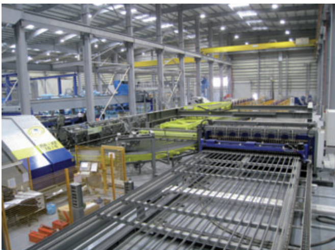
Mesh Welding Line
