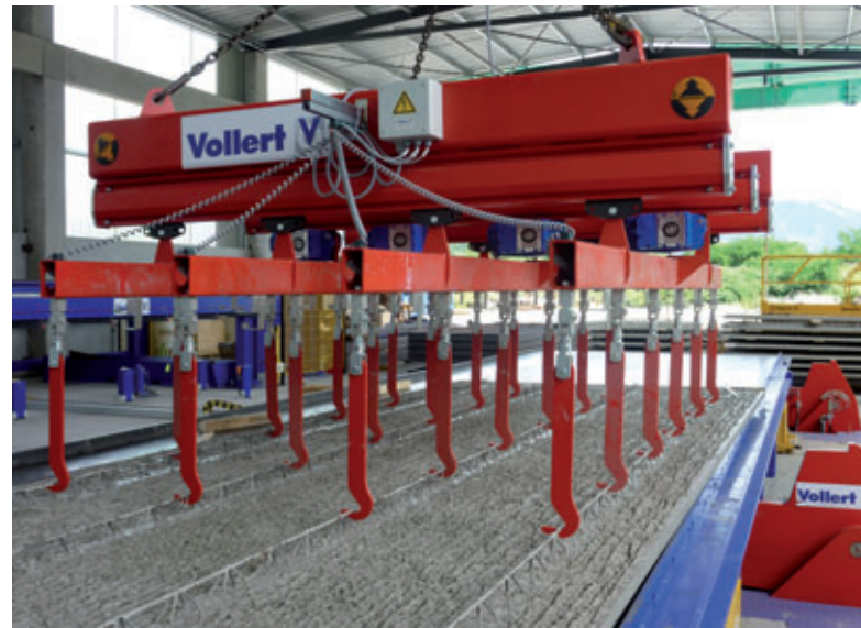
Lifting cross beam for horizontally lifting off the floor slabs
