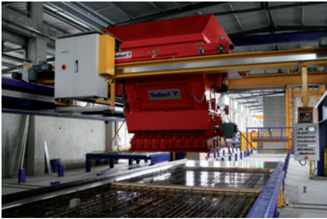
3.3 m 3 concrete distributor with screw discharge
