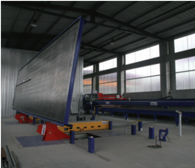
Overhaul tilting table for vertically lifting off the double walls
