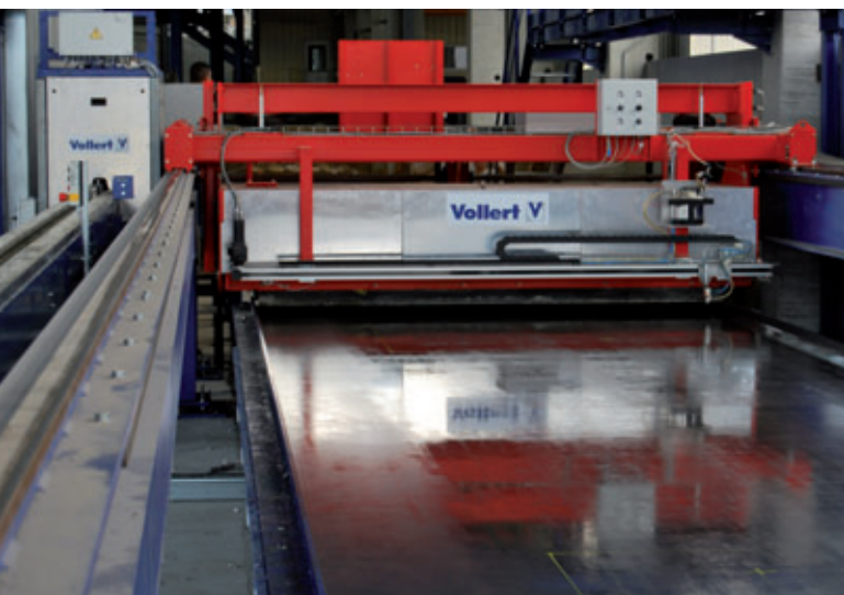
Cleaning, spraying release agent and plotting in one unit
