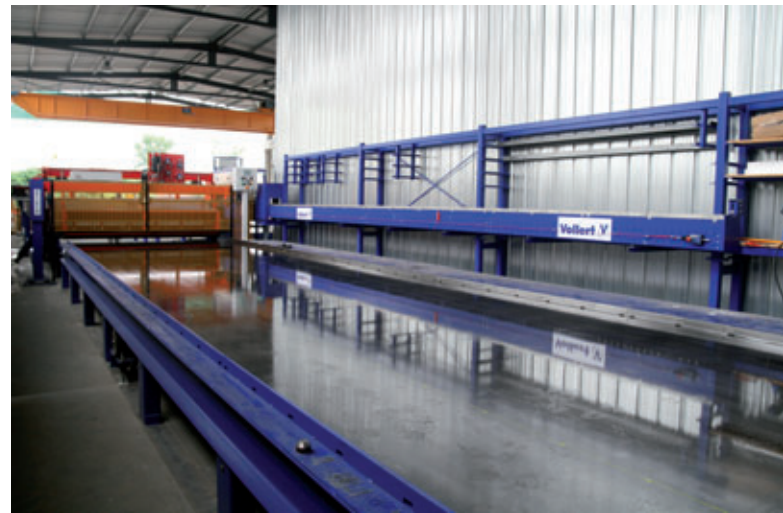
Workplace system with integrated formwork transport for storing and positioning formwork and built-in parts.
