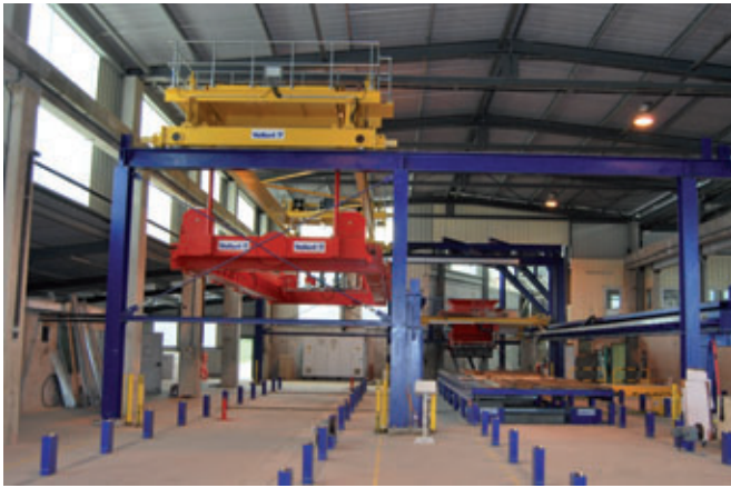
Pallet turning unit for the production of double walls
