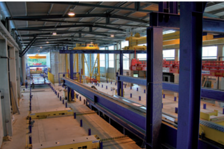
The layout of the pallet circulation plant makes efficient use of space
