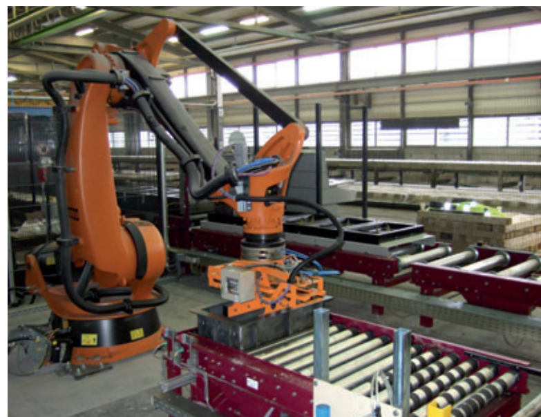
At the completion station, the cleaned, oiled frames are once again positioned on the boards with the models by means of an industrial robot
