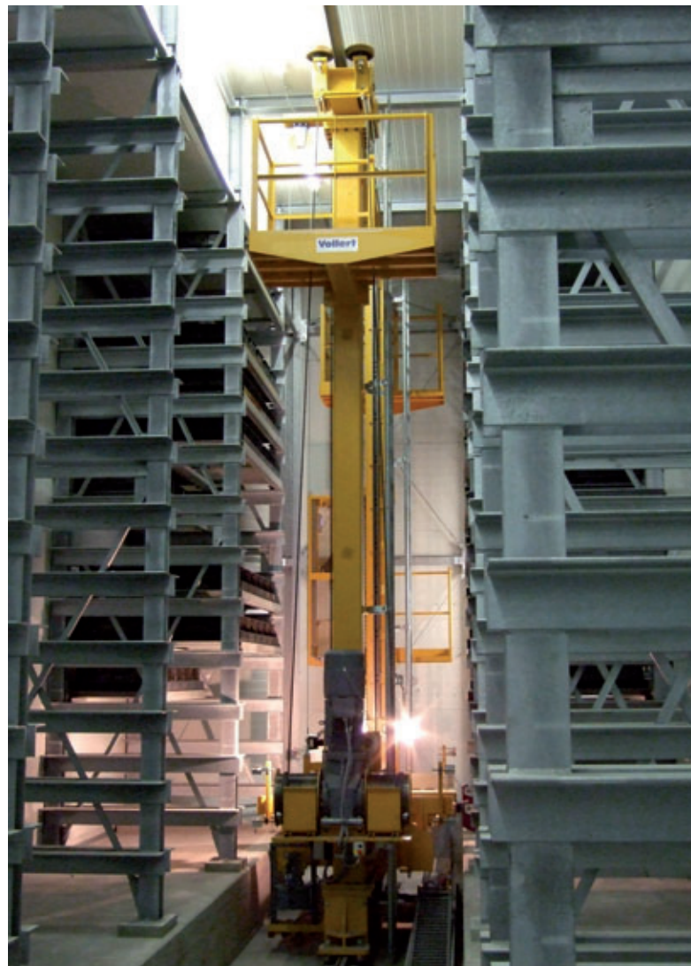
The concreted blocks are brought via roller conveyors to an adjacent high-rack storage area for curing
