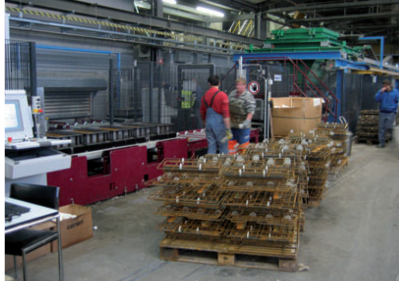
The board with model and frame is brought to the employee at both manual workstations for inserting the reinforcement
