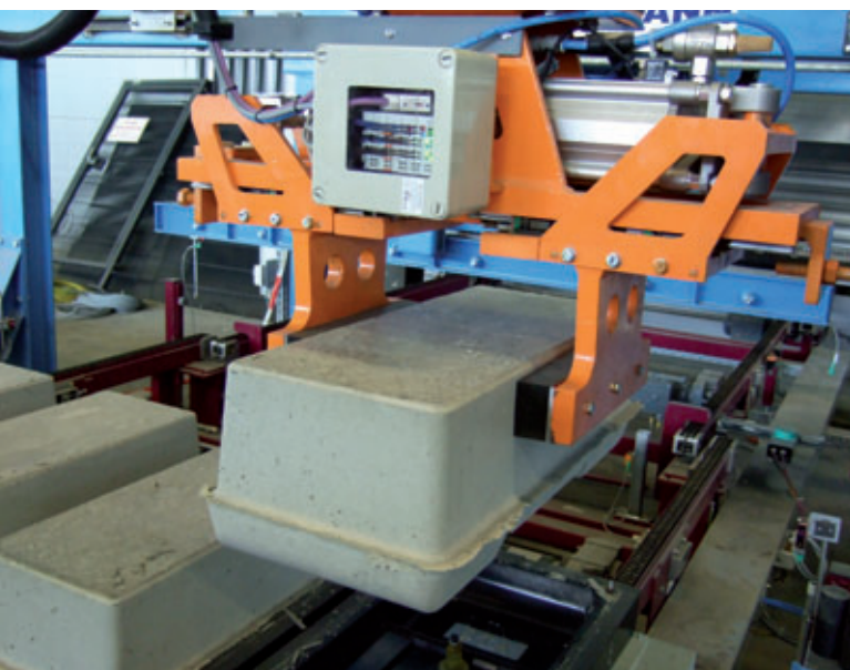
The blocks are removed from the board with the aid of an industrial robot
