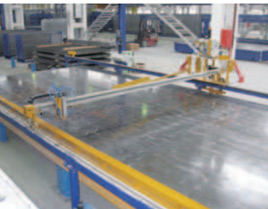
Plotting element contours including assembly parts on a pallet at a scale of 1:1
