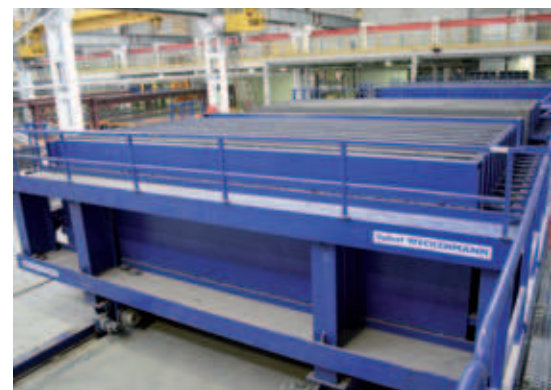
In two enclosed neighbouring bays, a total of 9 battery formwork systems have been set up
