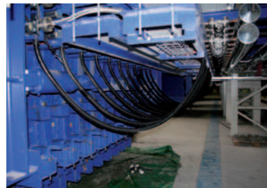
All panels are equipped with heating coils which are supplied with thermo oil via a central heating unit
