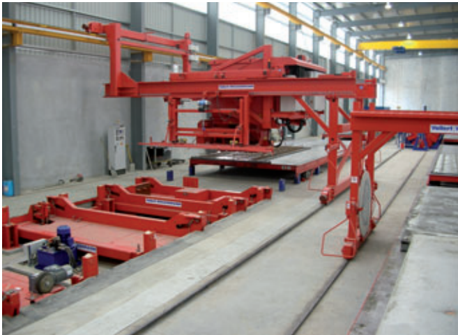
Fig. 16: Concrete and compacting station
