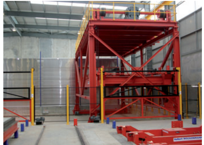
Fig. 17: AS/RS with curing chamber
