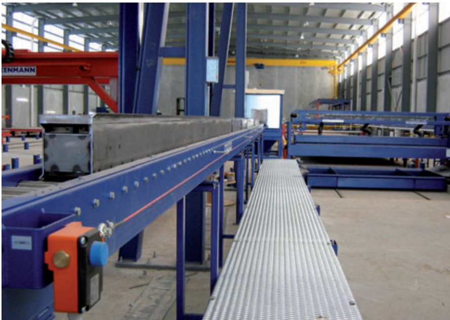
Fig. 11: Solid wall shuttering transport system
