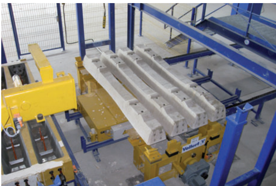
Concrete sleepers before final assembly
