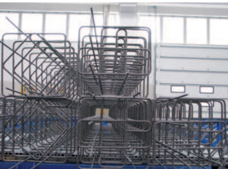
Fig. 31: Cages Produced on AWM Autobend
