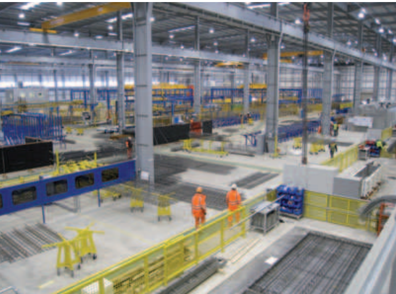
Fig. 35: Cage Assembly Area
