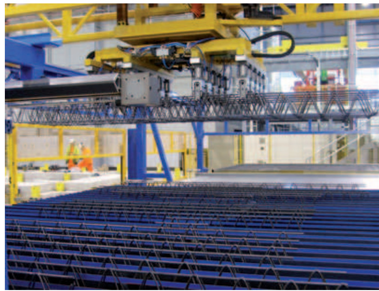
Fig. 34: Lattice Girder Placing Robot
