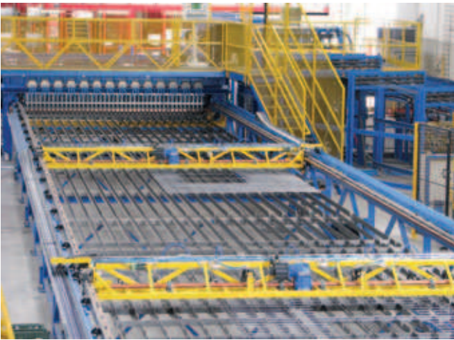
Fig. 29: Mesh Exit Bench and Pulling Carriages
