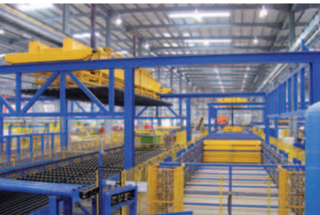
Fig. 30: Mesh Crane and Buffer Store
