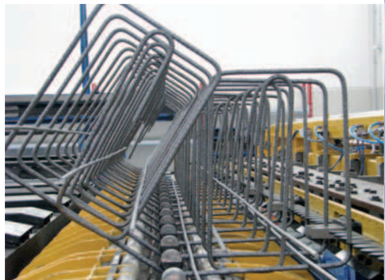
Fig. 32: AWM Autobend Closing Cage
