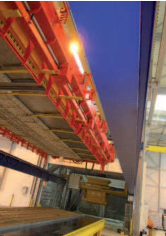
Pallet turning unit with pneumatic clamping system
