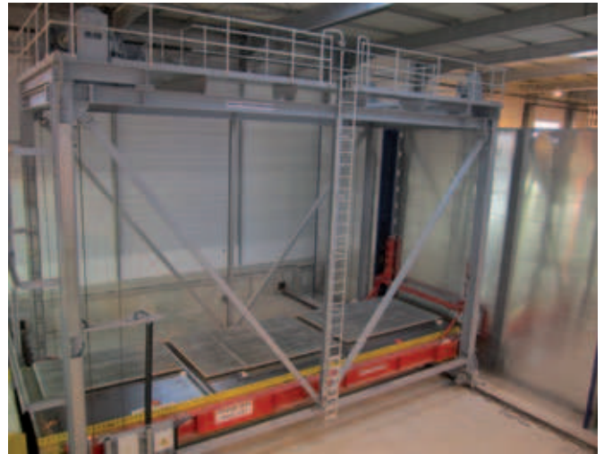
Storage and retrieval machine and curing chamber
