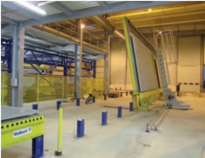
Circulation of the movable ladder in the area of the tilting table
