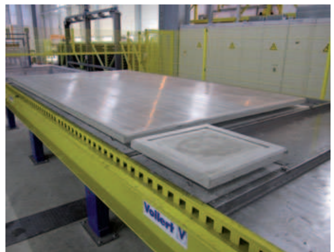
Double wall with form liners before demoulding
