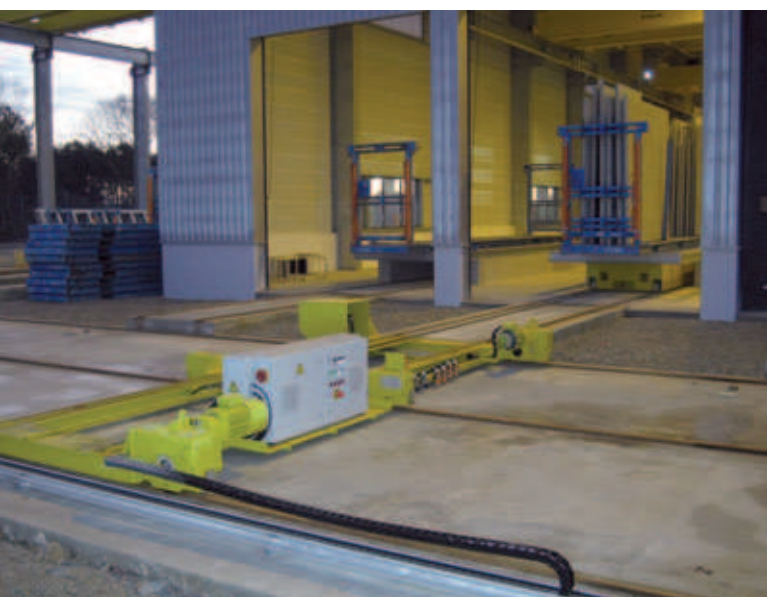
Run-off truck system for transport cradles and element stack
