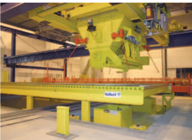
Concrete distributor and vibration station (front), the turning machine in the background
