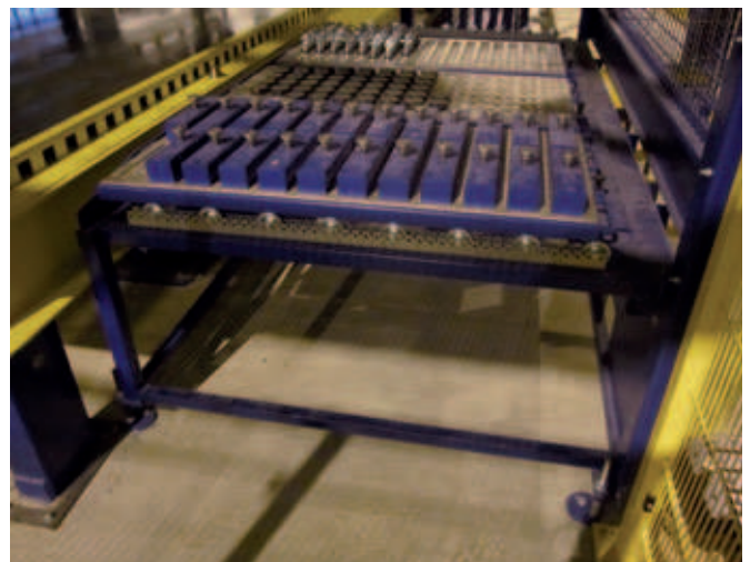
Storage for component magnets and magnet boxes in the robotic area
