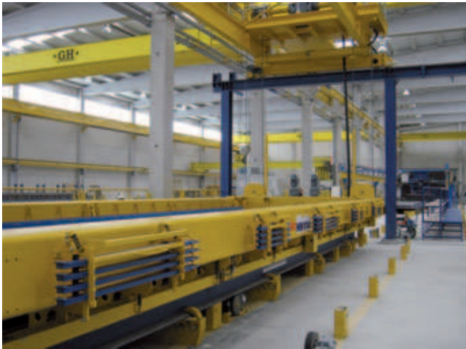
Turned-in pallet during the compaction procedure
