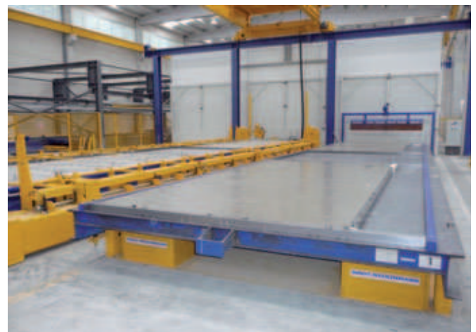
Situation after the installation of the turning machine and vibrating station
