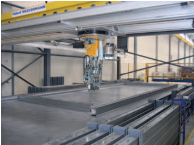
Formwork robot with magazine for solid wall formwork
