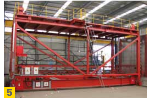
Automatic storage and retrieval system with curing chamber
