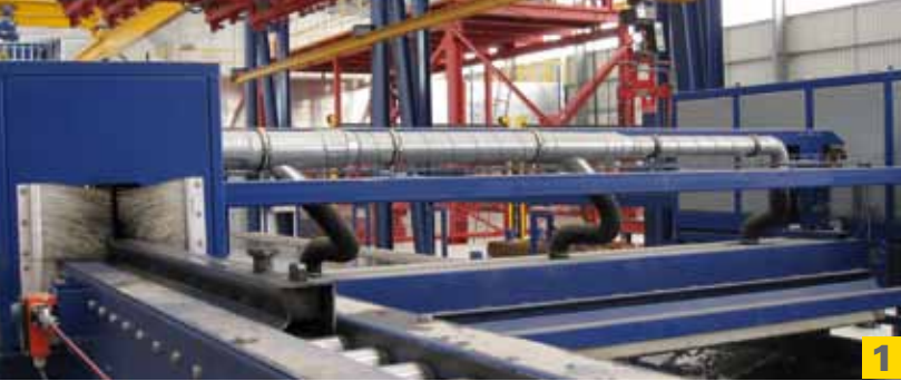
Cleaning of pallets and shuttering
