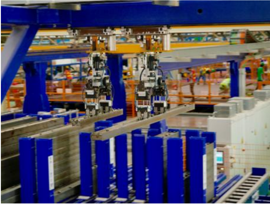
Fig. 1: A magazine robot with twin grippers stands for a simultaneous moulding and demoulding process
