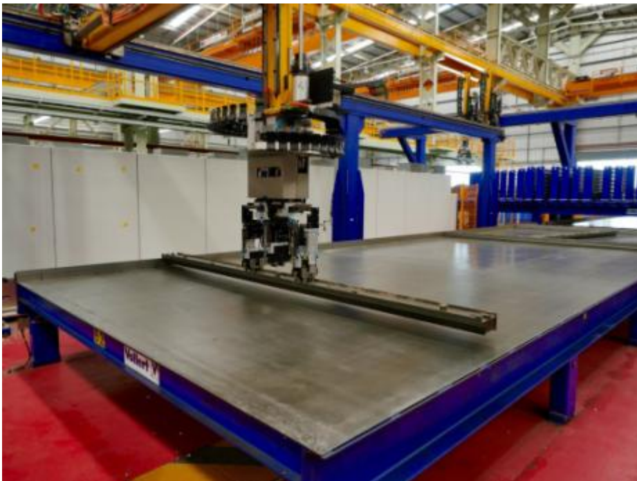
Fig. 2: Plotting the contours and positioning the shuttering systems is controlled via CAD/CAM and carried out by a state-of-the-art SMART SET shuttering robot
