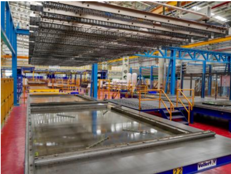
Fig. 4: The reinforcement and the lattice girders are then inserted via a fully automated AWM reinforcement system
