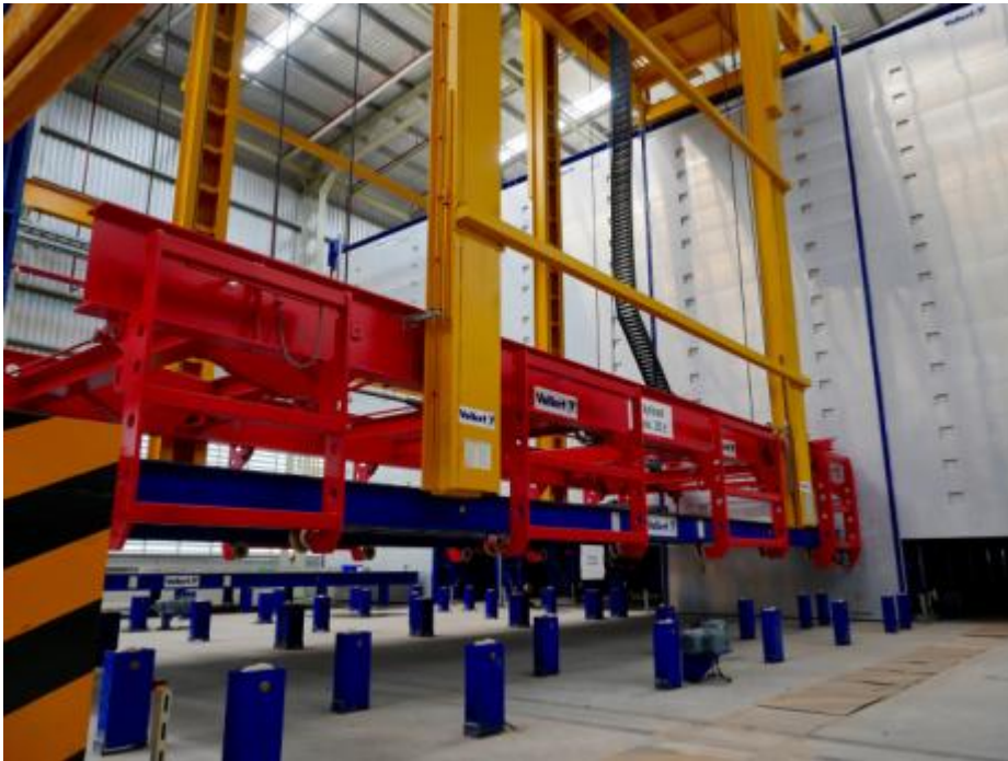
Fig. 9: The Vario CURE curing chamber consists of four encased rack towers featuring 16 pallet trays each
