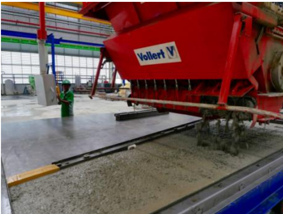
Fig. 6: The SMART CAST concrete spreader features a total of ten discharge screws for precise metering
