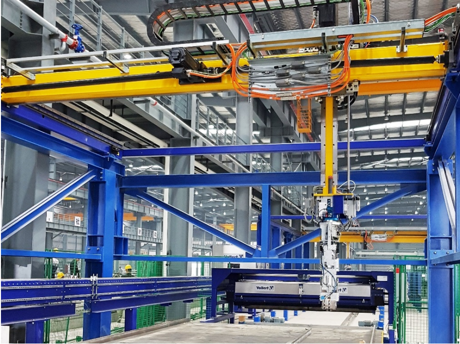
Image 2 Highly automated SMART SET shuttering and de-shuttering robots play a crucial role in terms of in plant productivity.
