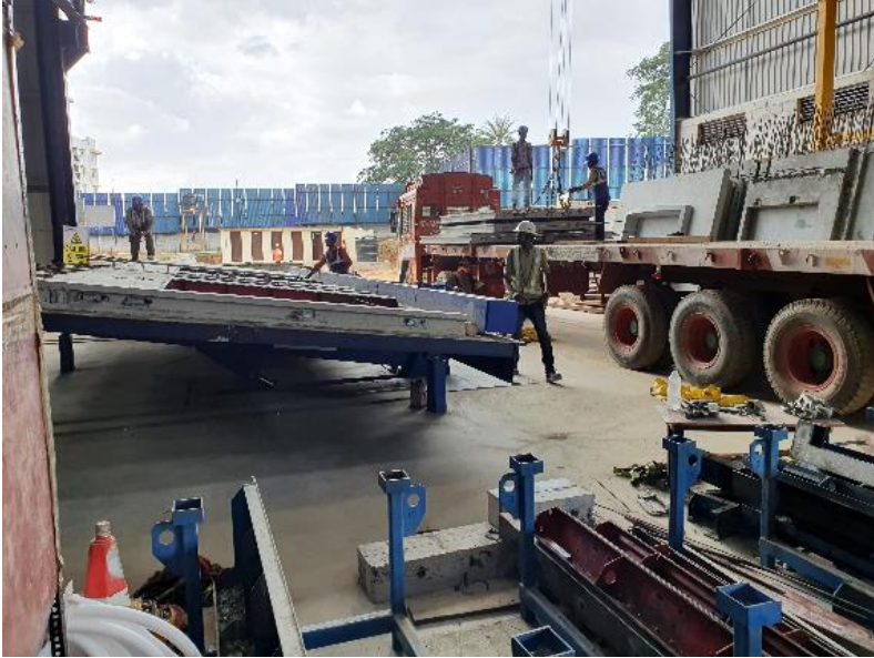
Image 7 A Vario TILT tilting station takes over the vertical lifting of the solid concrete parts.
