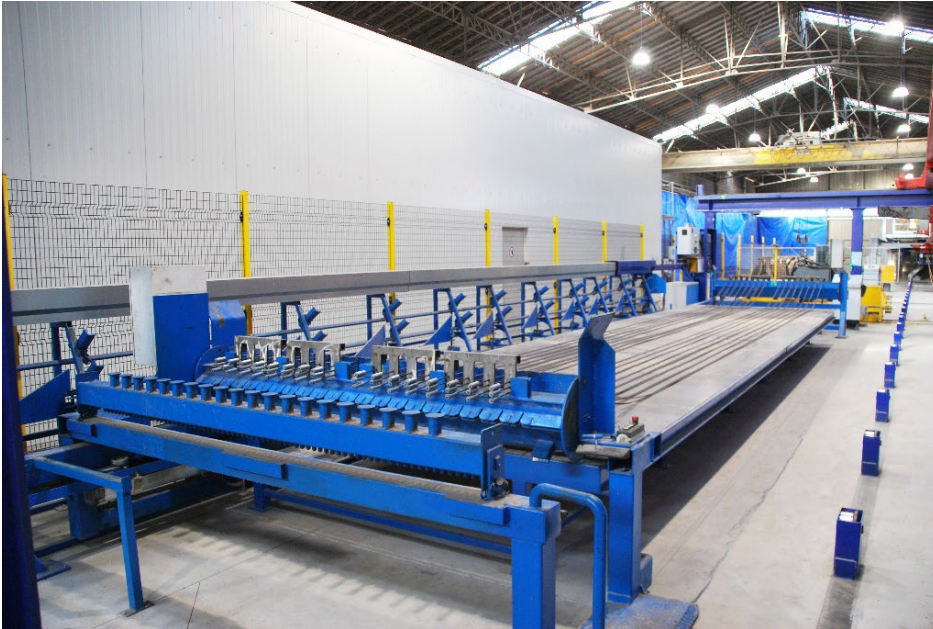
Image 1 Prior to the concreting process, the tension wire packages are prefabricated with sleeves.
