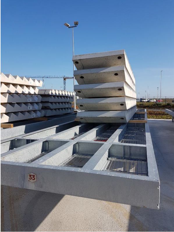
Image 4: A transfer platform then automatically transports the concrete element on transport racks to the open-air site and makes them available again on call for loading, optimally prefabricated.
