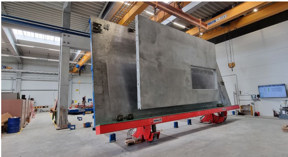
Image 11: Vertical lifting of the walls is performed by a VARIO TILT high-performance tilting station.
