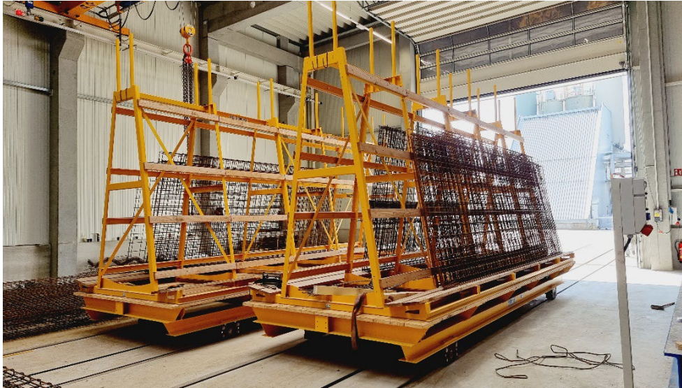
Image 10: Transport trolleys deliver reinforcement mats.
