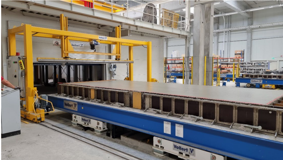
Image 6: A SMART COMPACT shaking station ensures optimum concrete compaction after the concreting process.
