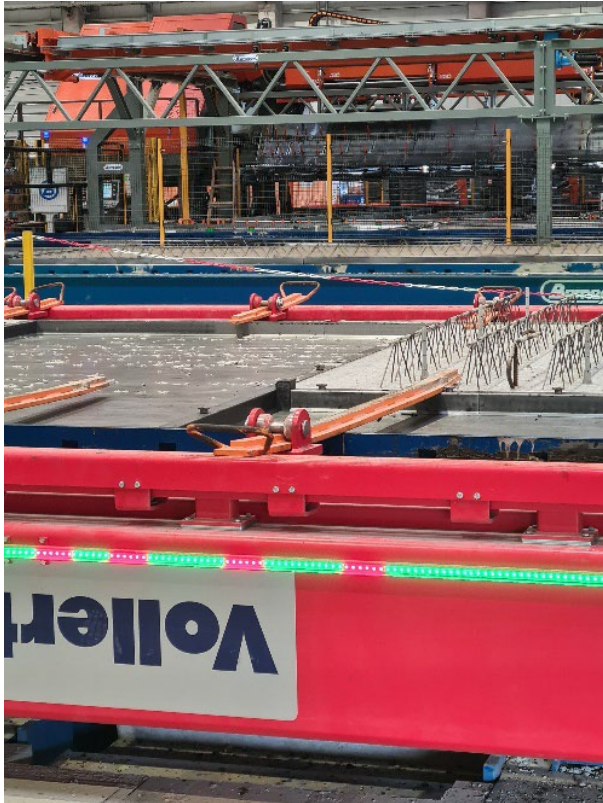
Image 7: An LED indicator bar on the long sides of the turning device shows the adjustment positions where no clamping arms must be inserted.
