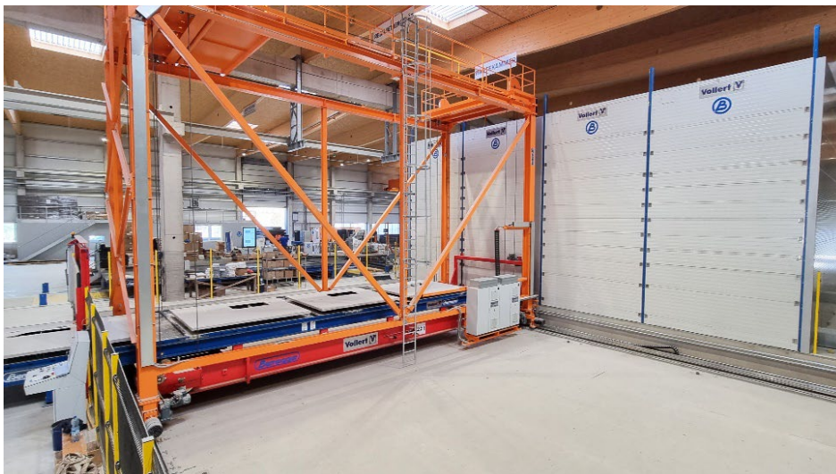
Image 8: An insulated VARIO CURE curing chamber with a special heat circulation system ensures an energy-efficient curing process.
