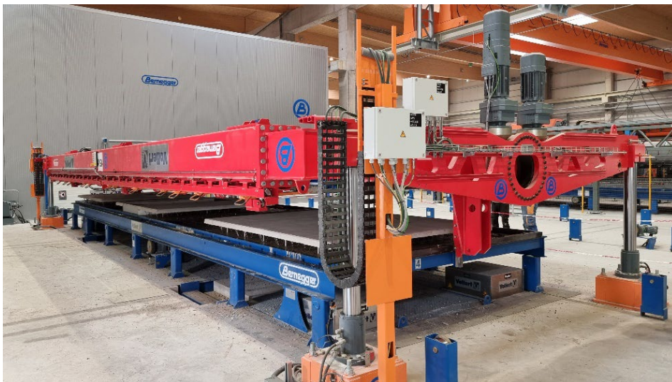
Image 6: A stationary VARIO TURN pallet turning device ensures a simple semi-automatic turning process in double-wall production.
