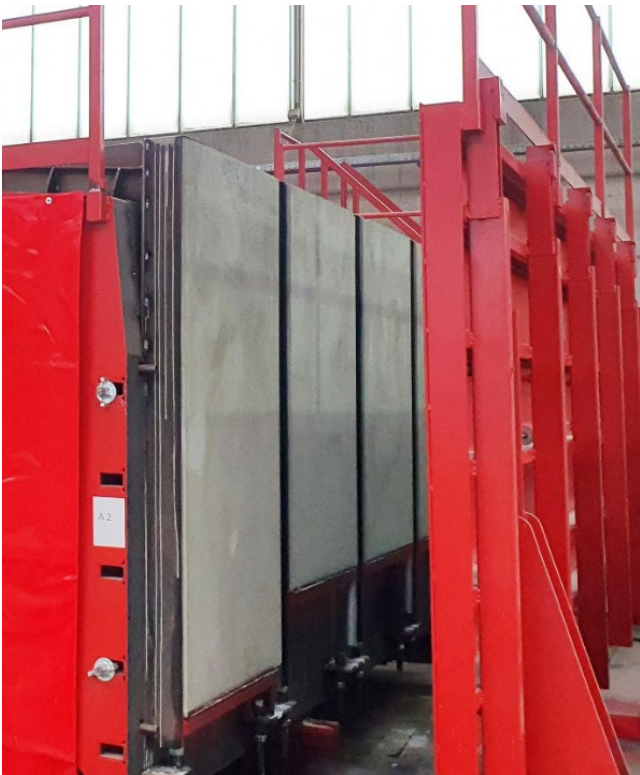
Image 4: The bricks are produced upside-down for outstanding surface quality.
