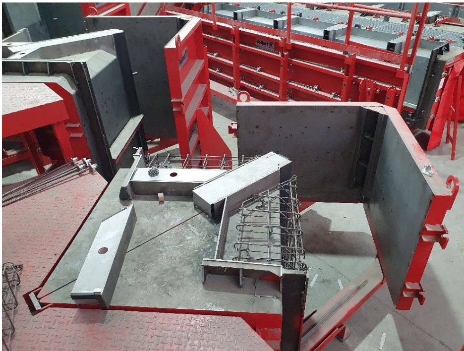
Image 6: The L-shaped side shutter is pneumatically moved on a diagonal to permit safe demoulding.
