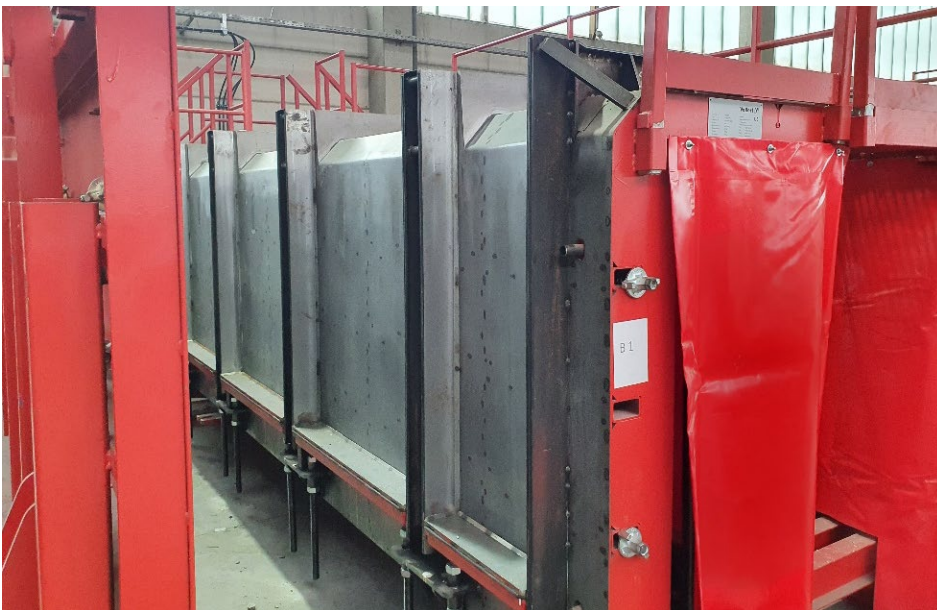
Image 2: Every formwork system can produce 8 L-elements with block widths of 99 cm and 2 L-elements each with block widths of 49 cm
