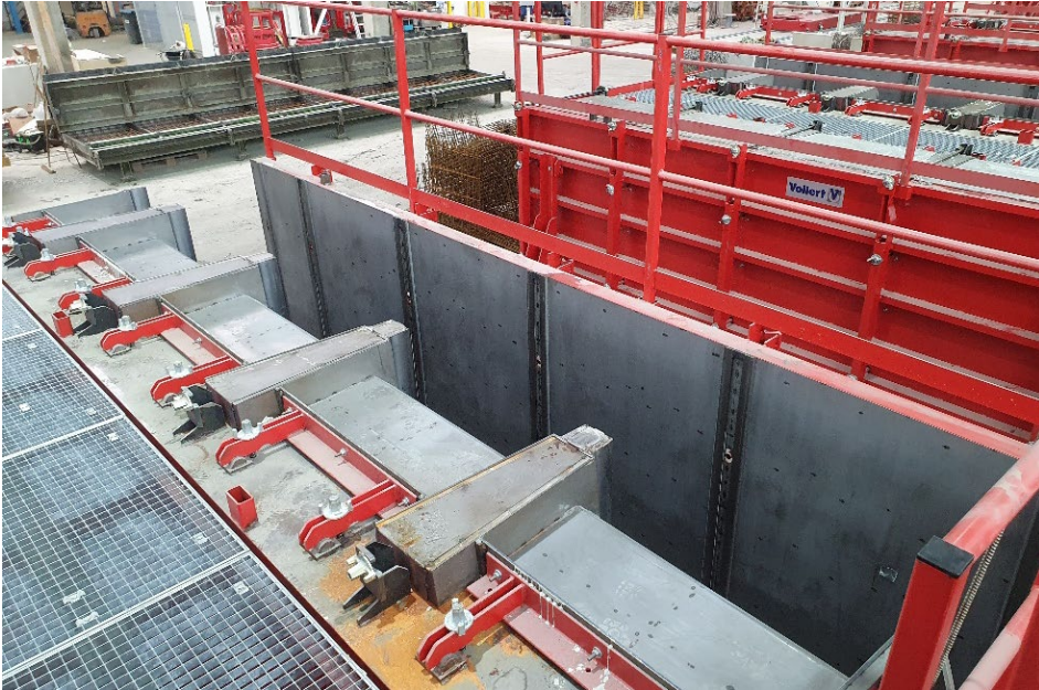
Image 3: The interim stops are divided due to the chamfer geometry.
