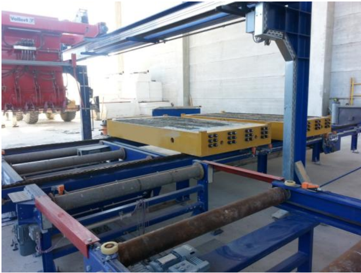
Fig. 4: The semi-automated concrete distributor fills the moulds precisely via electrically driven discharge screws.
