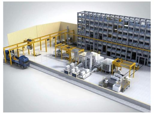
The Hydro Aluminium Rolled Products GmbH modernises its rolling mill in Grevenbroich for higher production quality. With smooth fully-automatic transport in the whole of the rolling mill and the loading and unloading of lorries, Vollert Anlagenbau ensures secure handling of the sensitive coils in litho quality. The high rack bay provides space for 336 aluminium coils with a total weight of 4,000 tons. (Graphic: Hydro)
