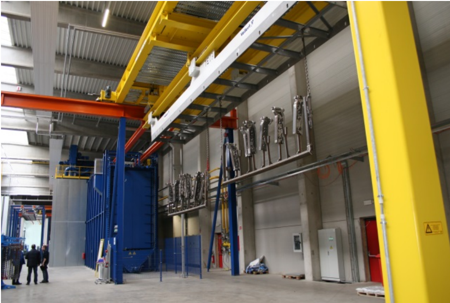
Image 2 Workpieces can be suspended individually or in a group on the transport units. A distribution manipulator (yellow) transports them to the various booths.
