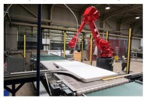
The ISO-MATIC 2.0 contours a wide range of insulation materials into the shape and size required with its 4,000 bar water jet and extremely high level of accuracy.
