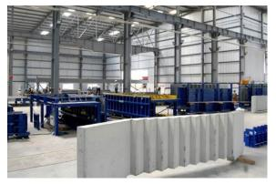
Complex, special-purpose elements and precast staircases are manufactured in India in addition to walls and slabs. Shuttering is carried out by a stationary solution from Nuspl.
