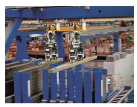
State-of-the-art magazining and shuttering robots operate with high turnaround times.
