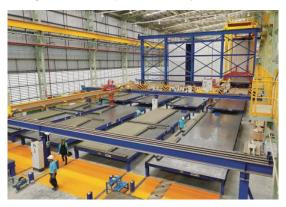
In Thailand, four power trowels are used to produce smooth mould surfaces. The VArio STORE rack operator then takes over the task of moving the pallets in and out of storage.
